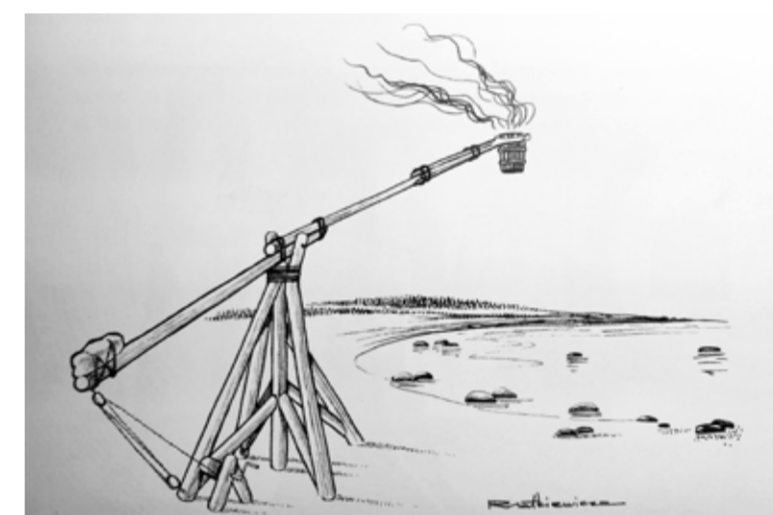
This is what the initial design of the Abruca leading light front beacon with a live flame in a steel cage might have looked like. Sketch by Roman Matkiewicz
