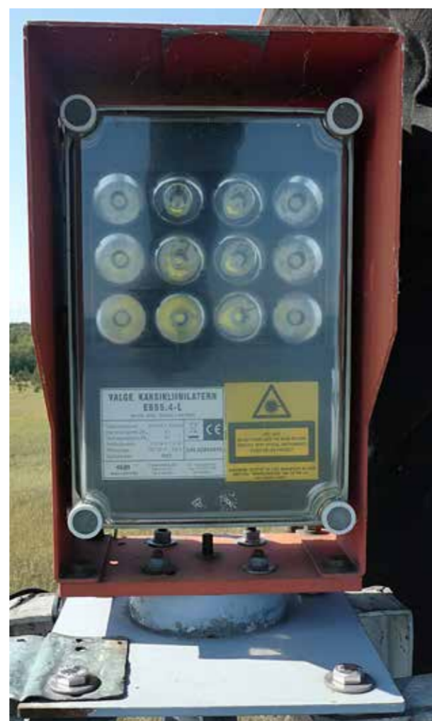
Abruca leading light front beacon's present range lantern (Sabik E855), photo from the year 2018, T. Vilu
