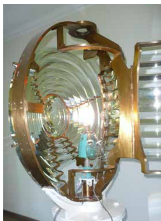
A 3rd order Fresnel catadioptric lighting device from the company Barbier et Fenestre Constructeurs installed in the year 1886, photo V. Laitus
